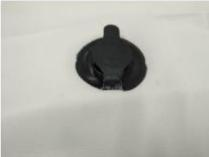
After eight hours, remove the patch and close the drain valve. Place the hot tub on an elevated spot and fill it with a small amount of water to check if the water is still leaking.
