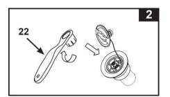
**IMPORTANT:** Never loosen or tighten the valve if there is water in the spa. Only use the supplied spa key to tighten the air valve. Do not tighten it too tight as this could result in a damaged valve.
