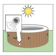
Through exposure to the sun and warm weather, the air expands and the pressure increases. The pressure relief valve allows the excess pressure to escape.
